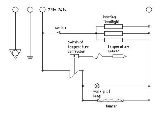
1. Power supply with single-phase 220V-240V, 750W-15KW
