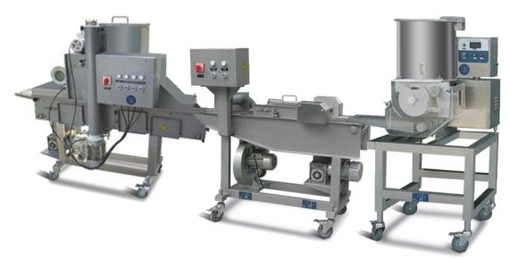
Mini Automatic Nugget Forming and Coating Processing Line (TT-ZJ200) : Forming Machine Patty 100-111 (TT-FM100) —> Battering Machine NJJ200-II (TT-BM200) —> Preduster (Flouring machine) SFJ200-II (TT-PM200)
